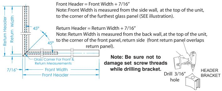
Take header bracket [F] (return panel side) and drill a 3/16" diameter hole completely through the end. Next insert wall plug(s) [P] into the holes that were drilled into each wall in step 2.
