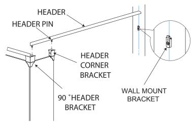
11 When aligning the header pins [H/B] with the headers [A/A1], make sure the headers [A/A1] are seated flush against the header brackets [E/F1/F]. Improper alignment will prevent fasteners from tightening easily in the following step.
