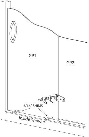
If interference exists, hinges can be loosened to adjust gaps. The gap should be 3/16" on each side of the door; 5/16" between the door and threshold at the highest point; door and panel(s) glass flush at top (glass not corner brackets). Re-tighten all screws after final adjustment. If hinge is scratched in the tightening process touch up paint may be used.
