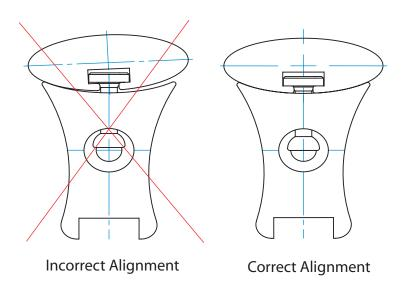
Place the four hubs [I] into each header bracket [F/F1/E]. The open side of the hub [I] **MUST BE** facing up and the header should be seated before tightening. If the hub [I] does not "bite", it may be necessary to push it deeper in the bore with a screw driver.
