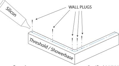
If no out of level conditions exist, cut u-channel [C1] to 71-1/4" (for a unit height of 74" which is standard height), or use formula (for custom unit height):
