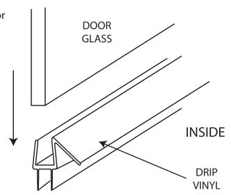
19 On the interior face of the glass, place a strip of low tack tape on the glass about 1/8" to 3/16" away from edge of the u-channel both vertically and horizontally. Run asmall bead of silicone along this edge. Next, on the interior, run a bead of silicone between the u-channel and the threshold and also between the u-channel and the wall. After completing, remove the tape before silicone sets.
