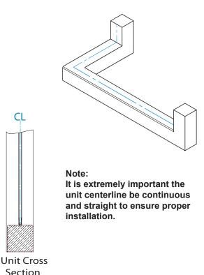
**2** Use a level to check the threshold for out of level conditions if the original measured conditions are not available. If no conditions exist, measure up each wall centerline a distance of 73" (for a unit height of 74" which is standard height), from the threshold, and clearly mark each location.
