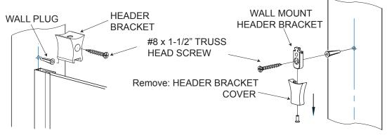
Temporarily place the 90° header bracket [F1] over the corner to ensure proper alignment of panels. Be sure that the glass fits into the bracket correctly. Remove the 90° bracket [F1]. Apply a piece of corner vinyl [L] to each of the three exposed glass corners. Now, tightly fit the header brackets [E/F1] over the vinyls.
