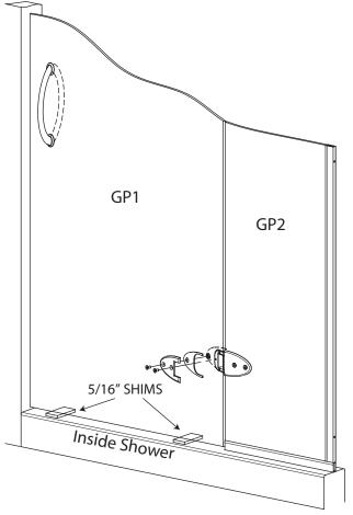
If interference exists, hinges can be loosened to adjust gaps. The gap should be 3/16" on each side of the door; 5/16" between the door and threshold at the highest point; door and panel(s) glass flush at top (glass not corner brackets). Re-tighten all screws after final adjustment. If hinge is scratched in the tightening process touch up paint may be used.
