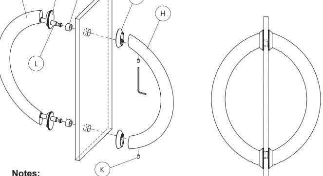
Make sure both handles are seated in their corresponding handle plates before tightening set screws.
