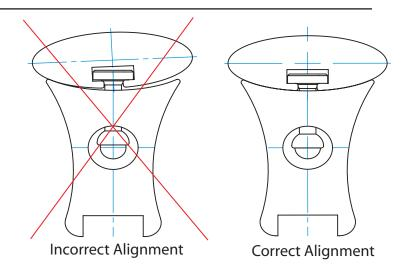
12 Place the two hubs [I] into each header bracket [F/E]. The open side of the hub [I] MUST BE facing up and the header should be seated before tightening. If the hub [I] does not "bite", it may be necessary to push it deeper in the bore with a screw driver.
