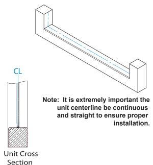
**2** Use a level to check the threshold for out of level conditions if the original measured conditions are not available. If no conditions exist, measure up each wall centerline a distance of 73"(for a unit height of 74" which is standard height), from the threshold, and clearly mark each location.
