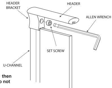
Note: Begin threading set screw [J] by hand, then carefully tighten with ball end of wrench as to not scratch the panel glass.
