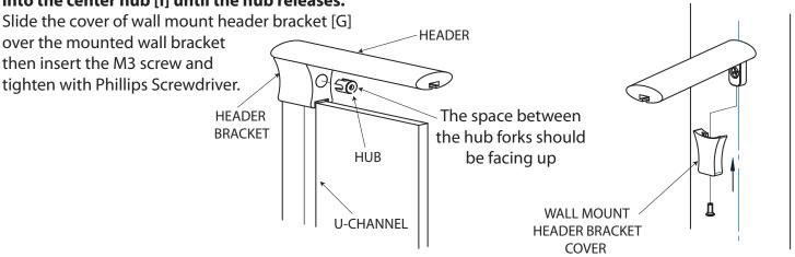
13 Verify the panel is plumb at the door opening and that the door opening measures 28-3/8" at the top, middle, and bottom of the door opening. Adjust the panel if necessary. Next insert the set screws [J] into the header bracket hole. The set screws [J] can be tightened with the allen wrench [M] provided. DO NOT install hole plugs [K] at this time.
