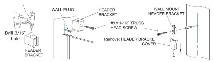
Note: Be sure not to damage set screw thread while drilling header bracket.
