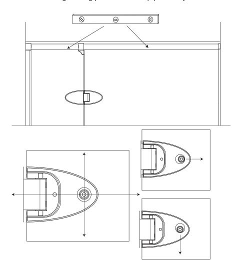
**NOTE: DO NOT install the plugs until completely** satisfied with the glass position.
