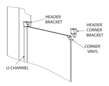
10 Slide one header pin [H] into end of the header [A]. Then align T-slot of the header [A] with T-lock of the wall mount header bracket [G] and slide it in. Line up the pins with the appropriate header bracket [F/E]. Drop the header pins into the header brackets [F/E].
