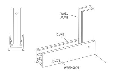
Wipe the shower walls and sill, the curb [A] and the wall jambs [B] with a clean, dry cloth to remove any dust or debris. Apply a 1/4" bead of caulk along the inside of both of the pencil lines marked in Step #2. Carefully replace the curb in the exact position marked. Caulk the inside of the curb ends where they meet the wall. Replace both wall jambs and attach to the walls with six #8 x 1 1/2" truss head screws [D].
