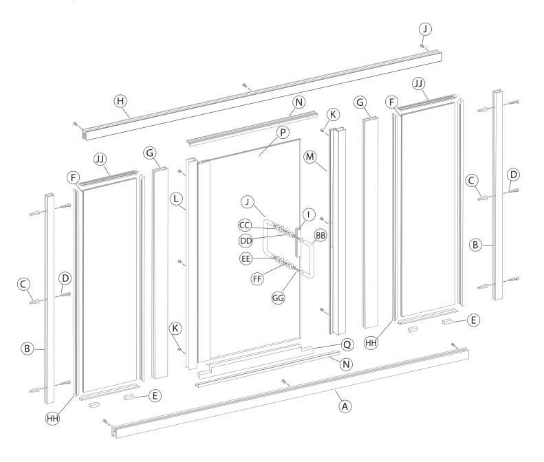
The frameless shower door panel is completely reversible and may be installed hinge-right or hinge-left. The door may hinge from the wall or from the center-post. Using the illustration, determine the correct position for the door in your particular installation. This instruction sheet depicts a hinge-right installation.
