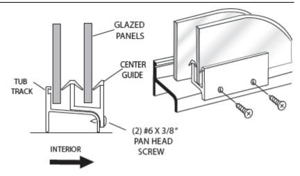
13 Neatly silicone each end of the tub track where it fits into the wall jambs as well as the seam between the wall and the wall jamb and the curb and threshold on the inside of the shower.
