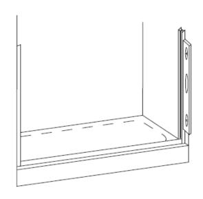
4 Before replacing the track, force a slight downward bow into it. This will ensure that the track fits tight to the threshold in the middle.
