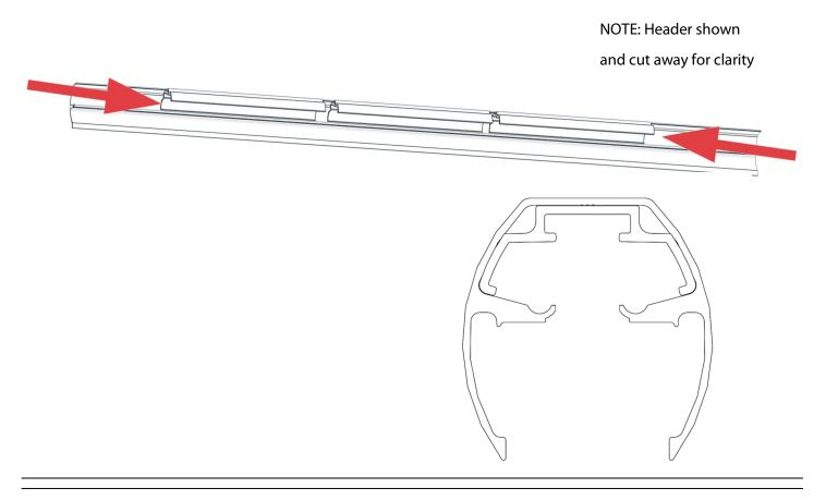
7 This enclosure is equipped with molded nylon T-Locks [F] for safety. When properly installed, the header is locked in the wall jambs and cannot be accidently removed.
