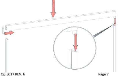
Slide the T-Locks into the header. Set the header down onto the wall jamb with the T-Lock fitting into the space behind the wall jamb.
