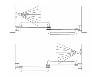
2 Measure the wall -to-wall opening along the center of the threshold at the bottom. Cut the Bottom Track (W/ Vinyl Silencer) [B] 1/16" short of that dimension.
