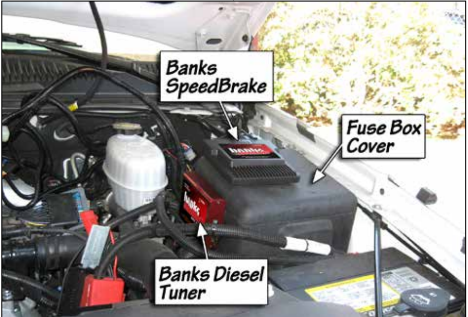
Figure 7 Placement of Banks Tuner on side of the Fuse Box.
