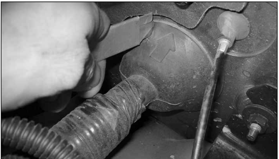
Figure 5 Driver Side Firewall, Rubber Grommet
