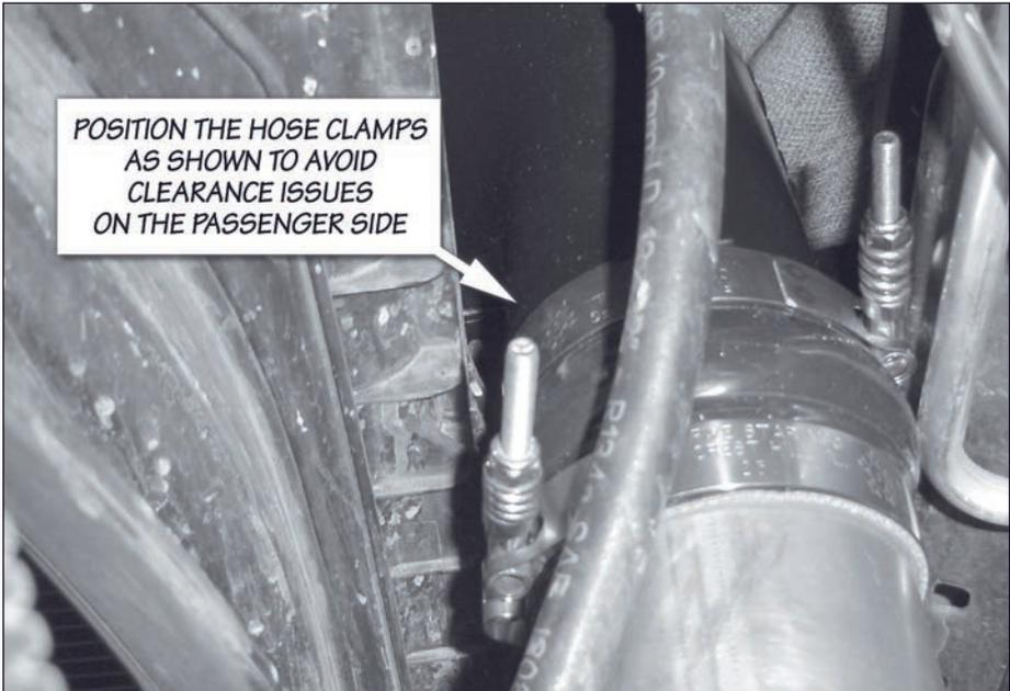
**Figure 8** Orientation of the Hose Clamps on the driver side.
