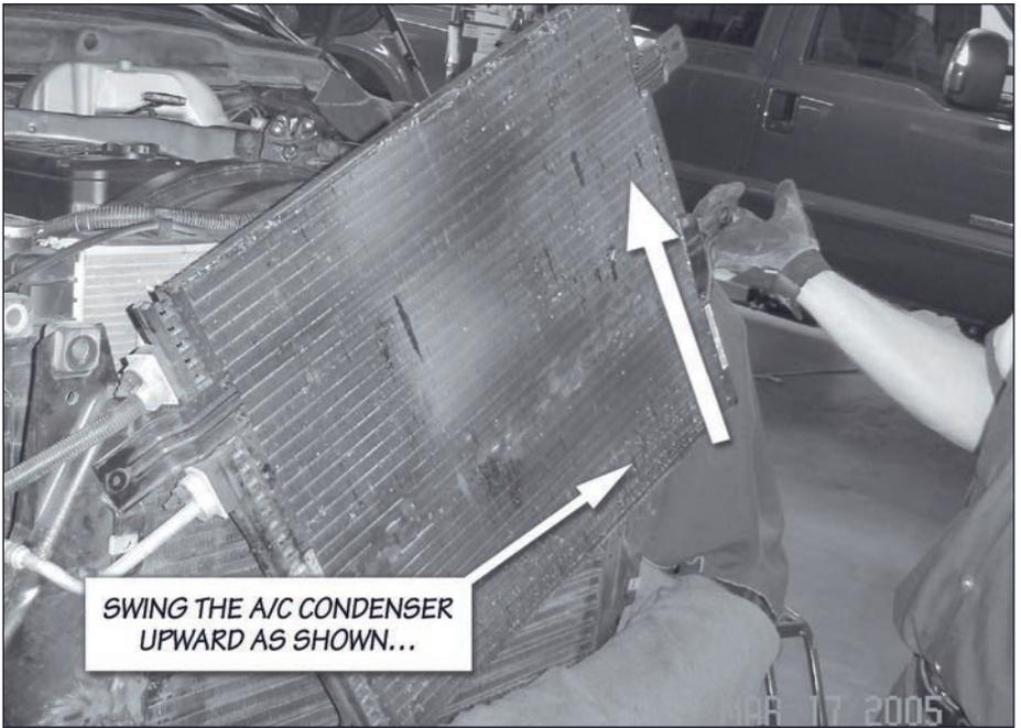
**Figure 6** A/C Condenser Removal Procedure
