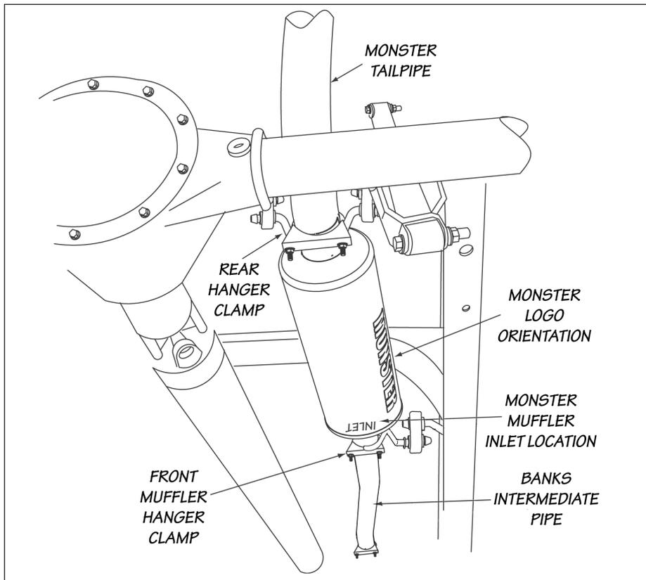
**12.** With the exhaust positioned properly, begin to evenly tighten the clamps starting with the ones closest to the front of the vehicle and working your way back. Torque the exhaust clamps evenly to 35 ft-lbs. Make sure that each slip is fully inserted (+/-1/4").
