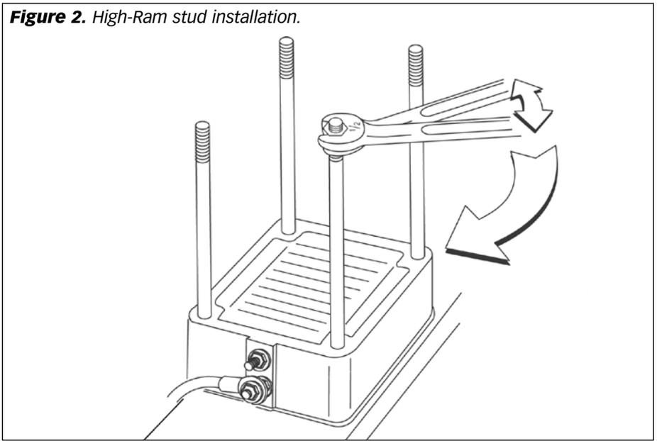
**13. CAUTION: The High-Ram/ Monster-Ram studs have different threads on each end. Make sure the M8 ends go into the engine intake manifold.** The shorter studs are placed inboard closest to the valve cover. Apply the supplied thread locking compound to the M8 threaded end of the studs. Hand tighten the studs to the intake manifold.
