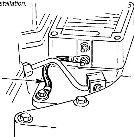
**9.** Install Banks driver side boost tube. The driver side tubes use a 3.5 inch diameter hump hose and Spring loaded clamps at the connection to the Banks Monster-Ram and re-use the factory hose and clamps at the CAC. Keep the hose clamps loose until the Monster Ram is installed. Cover the opening of the boost tube to prevent foreign objects from entering the boost tube during the installation.
