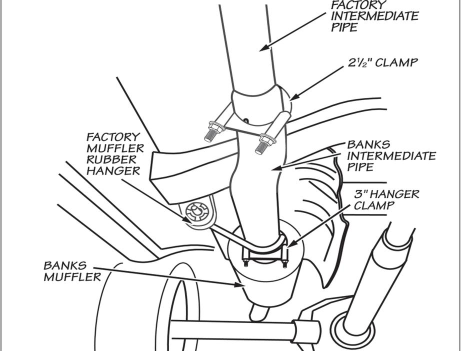
**6. For Ford Raptor models only,** the factory hanger in front of the muffler will need to be moved forward. Loosen and remove the bolts on the factory hanger and remove the Clip-on-nuts. Install the clip-on-nuts to the next forward set of factory holes. See **Figure 5**. Re-install the hanger using the factory hardware.
