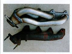
The Banks TorqueTubes are manufactured from 409 high-ductile stainless steel. The alloy is specially suited to handle repeated thermal cycling found in automotive exhaust applications. We measured the beefy flanges to be almost a half-inch thick, so warping at the head should not be an issue.
