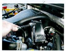
With the MAF sensor transferred to the Banks intake tube, it was installed using the factory throttle body gasket. The kit comes with attractive stainless bracketry to hold the intake in place.
