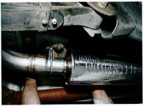
12 The Banks muffler is much more compact than the factory muffler and opens up a good bit of space under the bed. Our only comment on the muffler position is that we'd like to see it tucked up just a bit higher for off-road clearance.
