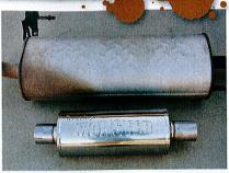
Ironically, the Monster muffler is dwarfed by the huge factory muffler. The Banks unit is a compact muffler with a polished stainless body.
