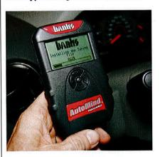
14 The Banks Power Pack kit comes with the AutoMind scanner/programmer. With it, the user can choose from six program options based on gas octane in use and the expected use of the truck. Custom settings allow the user to specify the speed limiter, rev limiter, tire size, transmission shift points, shift pressure, axle gear ratio, and engine fan activation temperature. The unit can also read and clear OBD diagnostic trouble codes, and can perform some data logging of sensor data.
