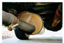
Moving downstream, we crawled under the truck and started loosening the factory tube clamps to pull the muffler and tailpipe off. The Banks Monster Exhaust replaces the tubing behind the Y-pipe with mandrel-bent stainless steel.
