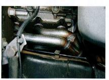
Here's a photo showing the driver side installation complete. The stainless headers add to the look of the engine. The rear collector meets up in the same location as stock to mate to the stock Y-pipe with the catalytic converters.
