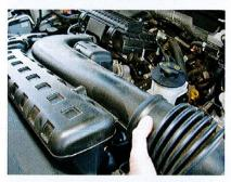
We started the installation of the air intake kit by unplugging and removing the MAF sensor in the stock intake tract, and removing the stock plastic intake tube and air filter housing. The Banks kit reuses a few small stock parts but the majority (of pieces) are replaced with upgraded components.
