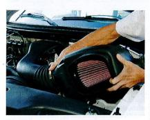
The new Banks filter element is a large, oiled type which is mounted into a new filter housing. The filter housing is attached to the new intake tube with a supplied rubber boot. The housing still draws air from the original hole in the inner fender, but also intakes air in the large opening shown here that resides behind the driver side headlight. The housing rides snuggly on two large grommets and the intake installation was complete.
