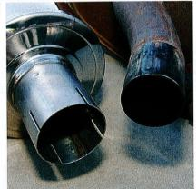
Here's where the monster part shows. The stock tubing is 2.5-inch diameter, whereas the Banks system bumps it up to 3.5-inch tubing aft of the Y-pipe. The muffler is a straight flow type with a perforated core.
