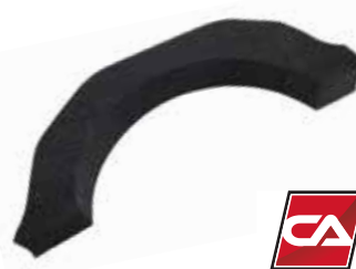
#X2475 1968-79 Transmission Tunnel Foam Collar Heat Shield
