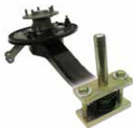
#X2480 1968-82 Trailing Arm Bushing Installation Tool
