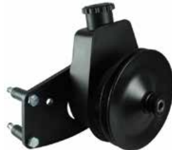
#MA18034 1965-70 PS Pump Upgrade - Small Block
