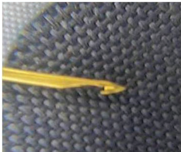
Figure 17. Close-up of the glover's needle tip that we prefer for thread removal.
