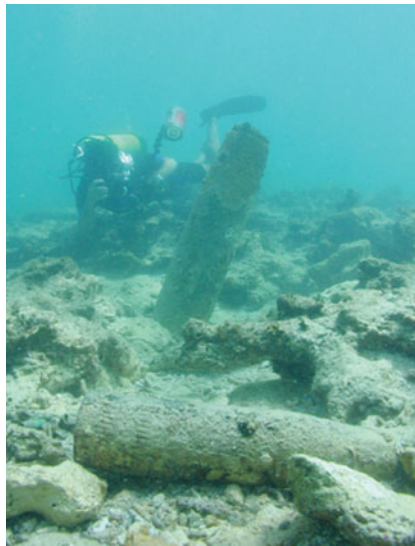
Figure 3.5 A 500 lb bomb in background; armed projectile in foreground (note rifling grooves); Vieques, Puerto Rico.
