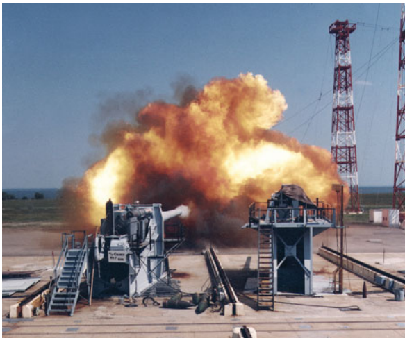
Figure 10.9 A 16-inch battleship gun is fired during proof tests on Dahlgren’s main range. The base’s large-caliber range is used to proof every naval gun before it is installed on a ship. “The 16-inch (406 mm) is the biggest and required this Potomac River location to have a 20 mile test range for the gun. Its range is 27 miles. Fishermen are ordered off the river for testing. The 16-inch was last tested for projectiles used on the Iowa in Desert Storm [8].”
