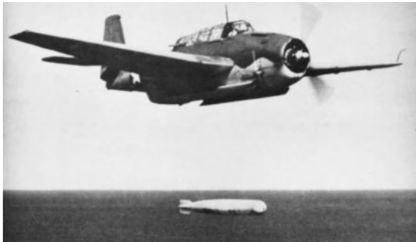
Figure 6.3 U.S. Navy Grumman TBF-1 Avenger dropping a torpedo in late 1942 or early 1943. An Avenger was seen over the Chesapeake per this entry: “In this rare photo (not the above photo)...She is predicted to turn left and land between the Chesapeake Bay... [6]”
