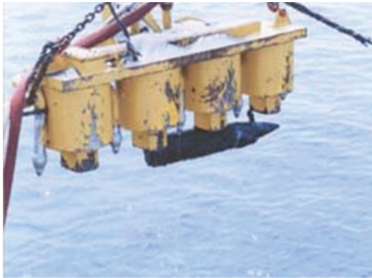
Figure 14.3 Electromagnetic underwater ordnance harvester. 5
