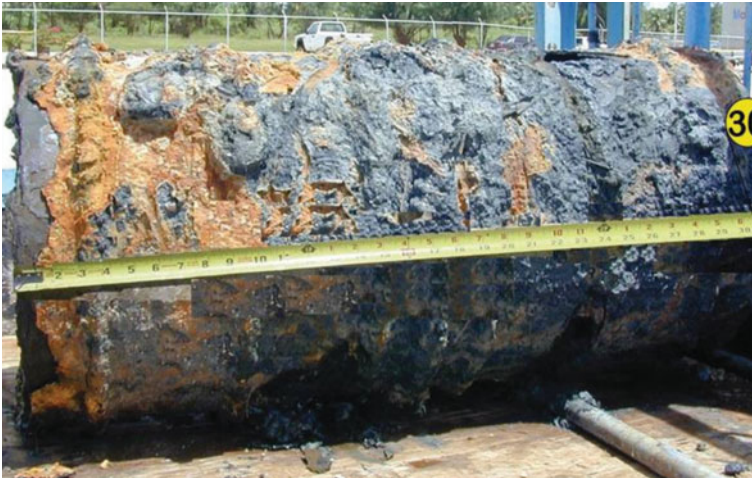
Figure 3.7 Fragmentation bomb from the Atlantic showing the complete rusting away of the casing. Source: AMPRO Consultants
