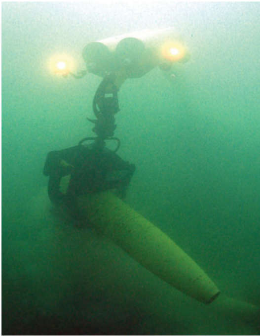
Figure 14.5 An ordnance harvester (invented by Jim Barton) on an SROV lifts a 500-pound high-speed, low-drag bomb, like the two shown in Figure 5.2 that were found in the shipping channel by Jim Barton and Richard Albright II.
