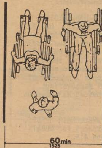
Fig. 2 Minimum Clear Width for Two Wheelchairs
