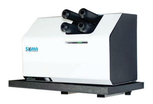
Wall mounted ultrasonic humidification for direct room humidification. High frequency vibrations of 4-16 transducers (1.7 MHz) producing extremely fine droplets delivering cool mist via variable speed fan out of the cabinet into the space with approximately 1M size droplets. Si6ma Ultrasonic humidifiers use 93% less power then electrode or infrared humidifiers.
