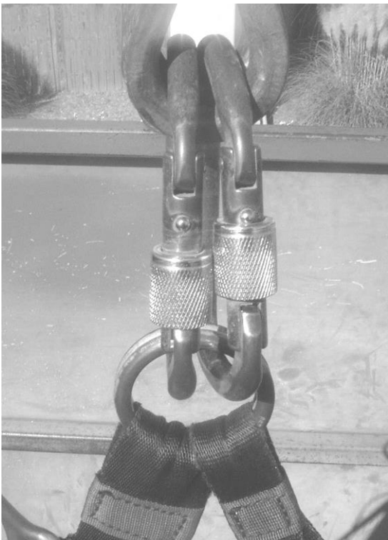
One gate unlocked
