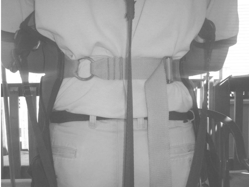
Good backstrap routing.
