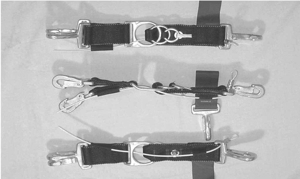
Good 3-Ring Assembly (3 different views).
