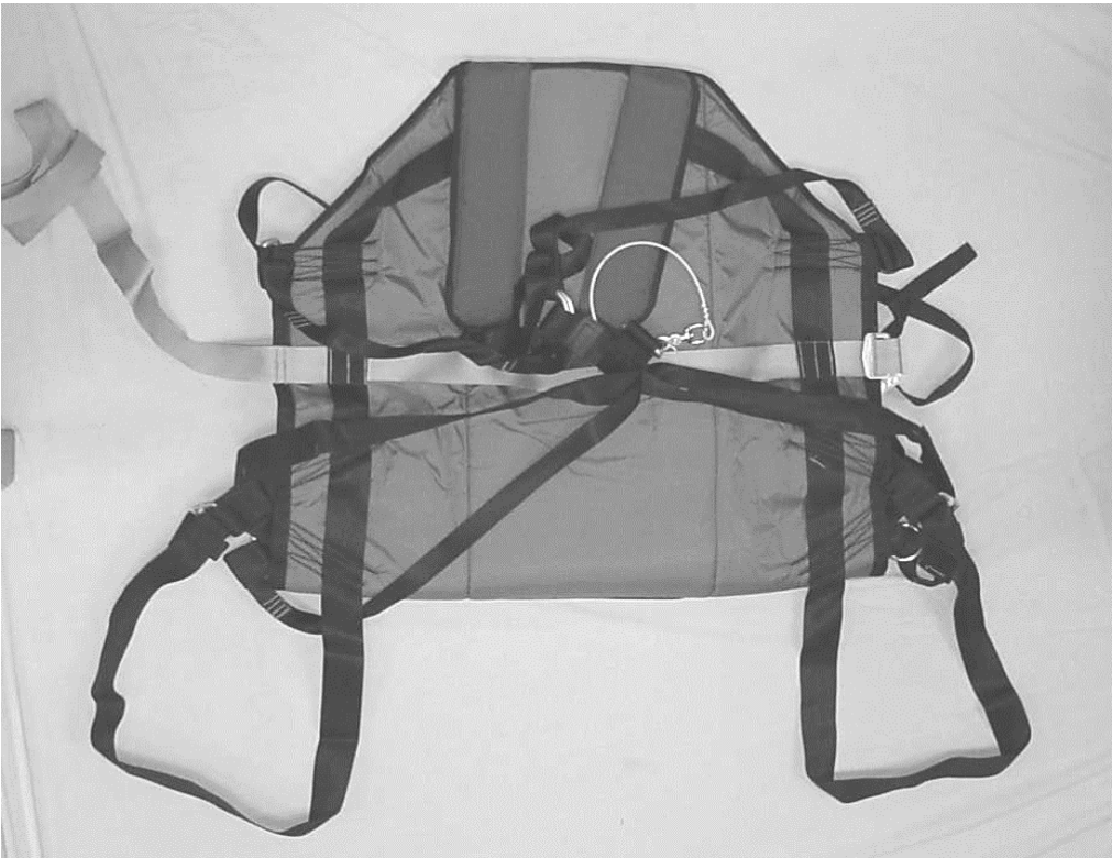
Bad Flight Suit Layout – suspension strap under leg loop.
