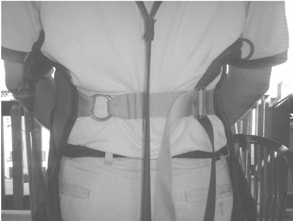
Bad backstrap routing (suspension strap under backstrap)
