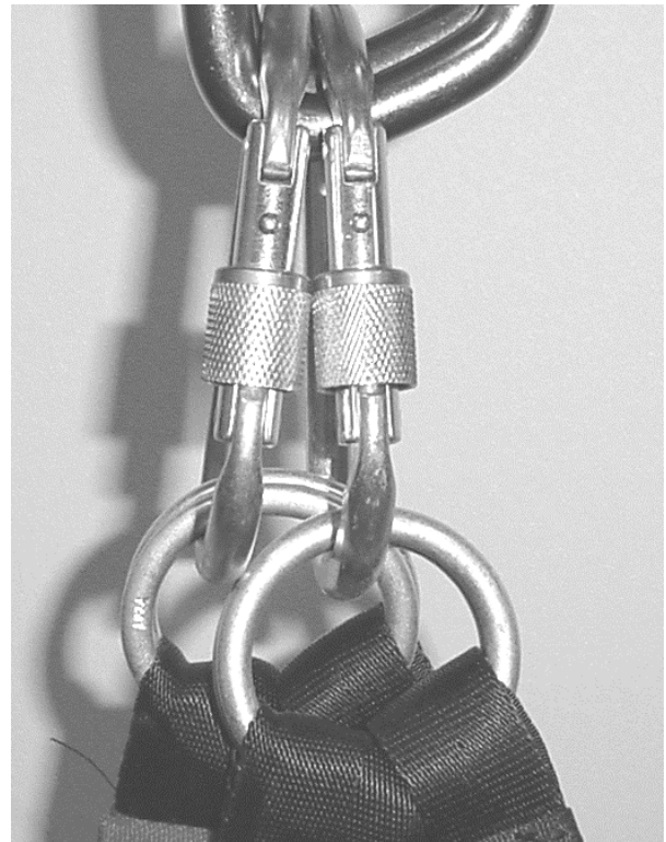
One suspension ring on only 1 carabiner
