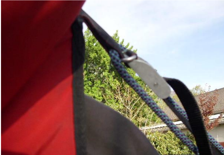
Photo showing secondary loop attachment at flight suit anchor buckle loop.
