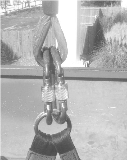
Both gates unlocked
