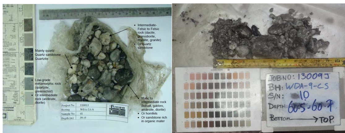
Figure 2 Photograph of sample from borehole WDA-2A-S at 39.45m below seafloor annotated with possible rock types and mineralogy, and sample from WDA-9-CS at 60.5m. (AG, 2013)
