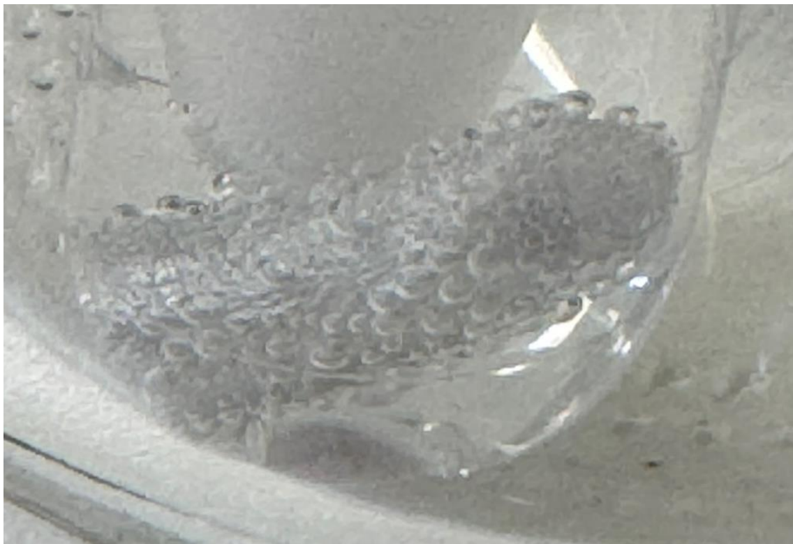
Figure 3: Rapid hydrogen evolution on the surface of the R2 alloy in CW.
