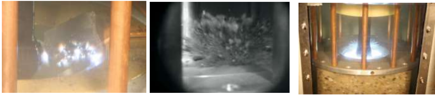
Figure 11 - Left- Electrical discharge traveling through the rock causing it to explode moments later photo middle, Right Demonstration first Drilling electrode.
