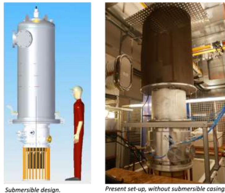
Figure 9 – Lab setup to test rock fragmentation, drilling electrodes and to obtain data on energy cost.
