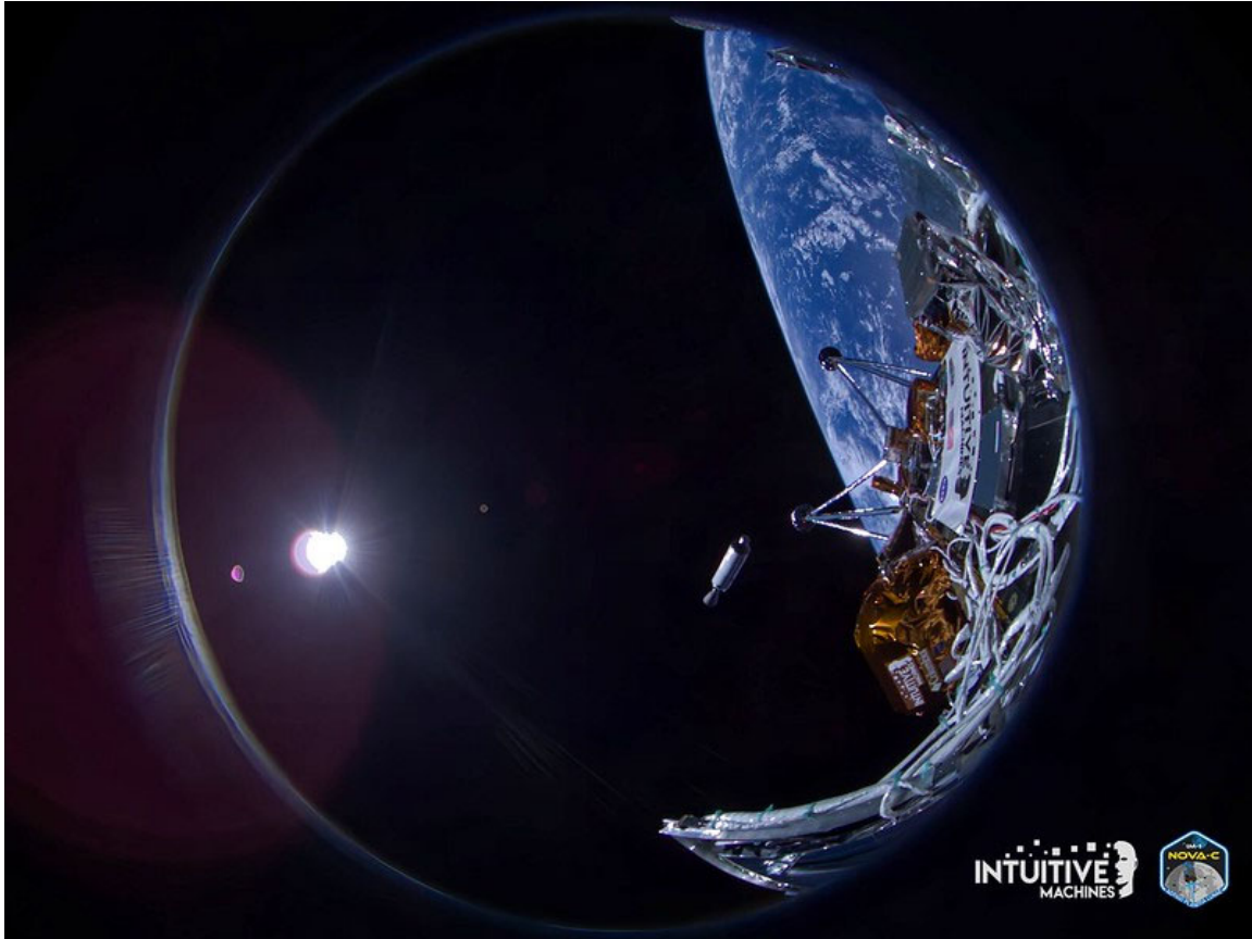
Figure 5. IM-1 Separation from the SpaceX Falcon-9 Upper Stage. The image illustrates the initial attitude being mostly engine-to-sun limiting solar array illumination.
