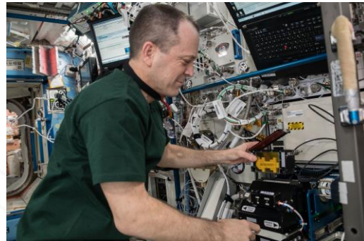
NASA Astronaut Ricky Arnold calibrates the Redwire Bone Densitometer aboard the ISS in 2018
