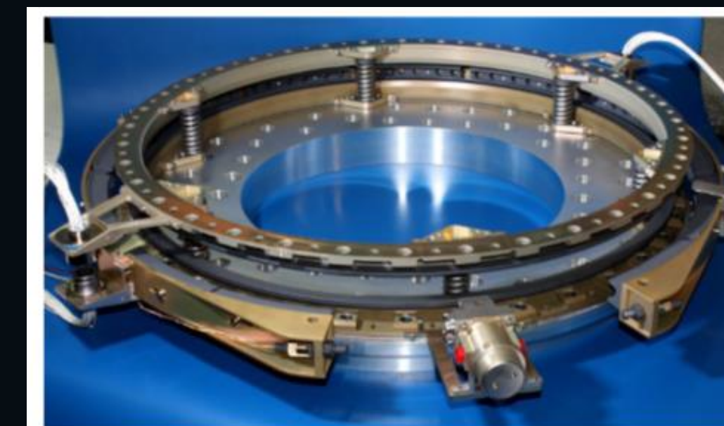
QwkSep 24 Low-Shock Separation System
