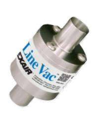
An eductor (or Venturi pump) uses compressed air to generate suction which will pull the granulate through the reservoir and then entrain it to be conveyed to the printer. An active feed mechanism will exhaust the motive air and force the granulate into the extruder using an auxiliary auger.
