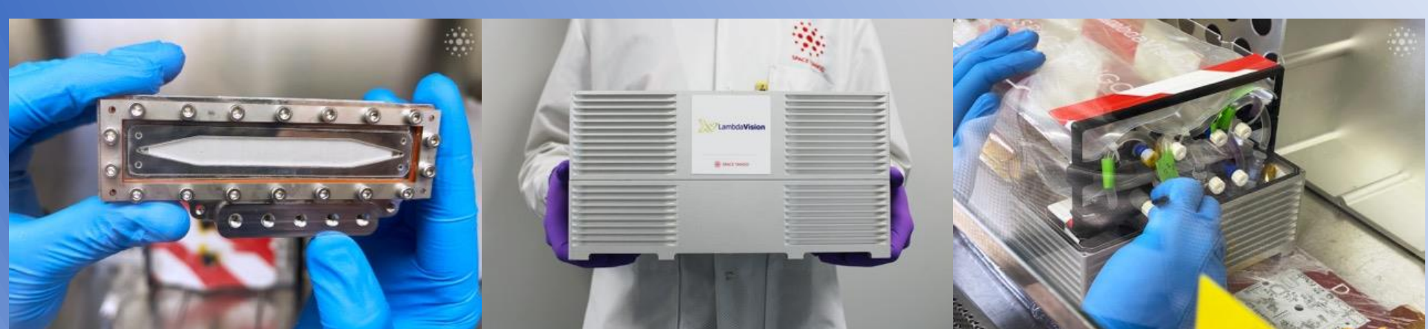
Figure 3. (A) LambdaVision and Space Tango developed a miniaturized and automated layer-by-layer manufacturing device for artificial retina production in LEO. (B) The sealed device is housed in a Space Tango Cubelab™, which contains bags for manufacturing solutions along with fluid handling hardware, sensors, and cameras.
