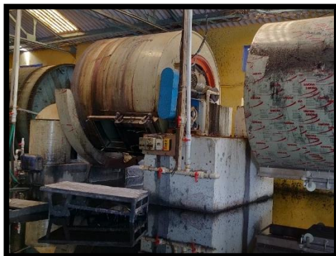
Fig 9: Mechanized Tanning Drums in TN
