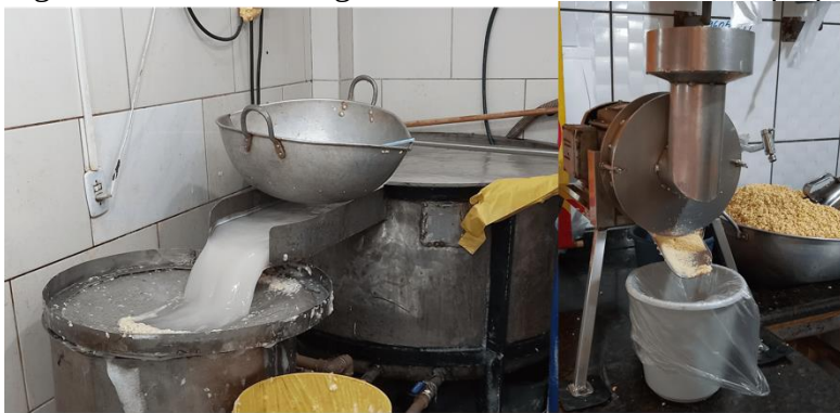
Figure 3 – Bean washing machine and electric mill for preparing ready-made batter
