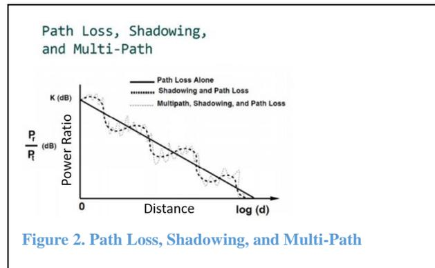
Figure 2. Path Loss, Shadowing, and Multi-Path
