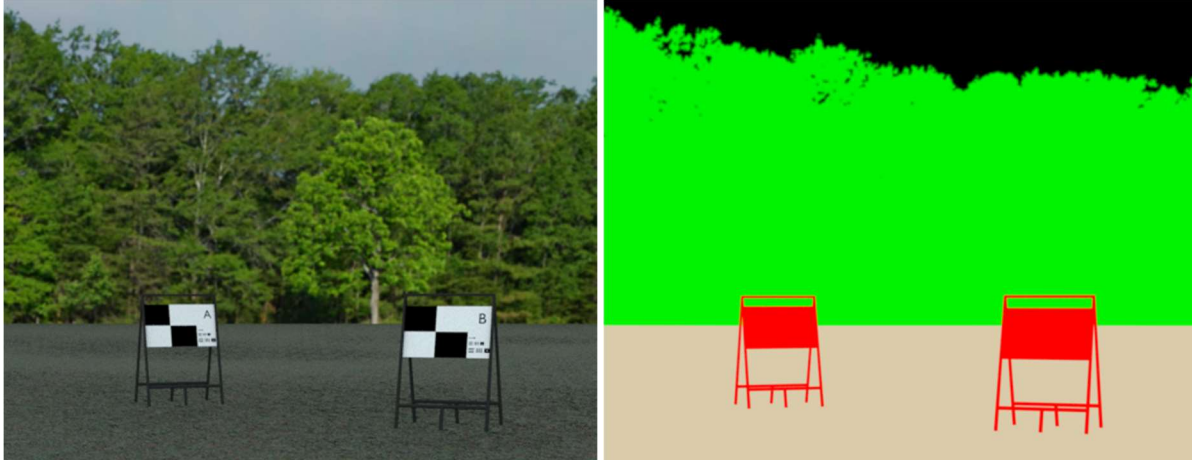
Figure 2. Illustration of Rendered Imagery and Corresponding Segmentation Mask
