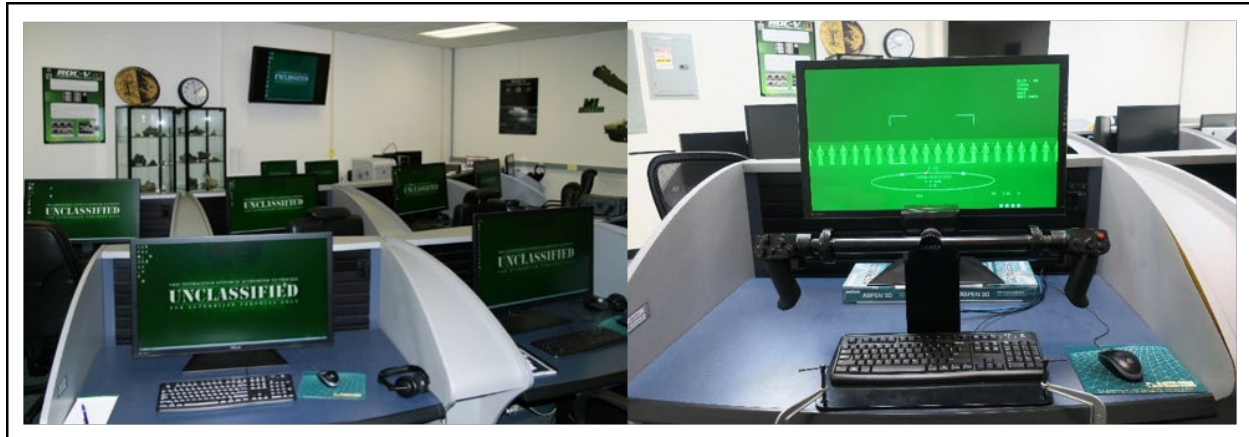
Figure 2: Perception Laboratory facilities and experimental configuration. The Perception Laboratory has 10 workstations for simultaneous testing (left). Controller grips were mounted to the desk and positioned in front of large, high definition 4K computer monitors (right).
