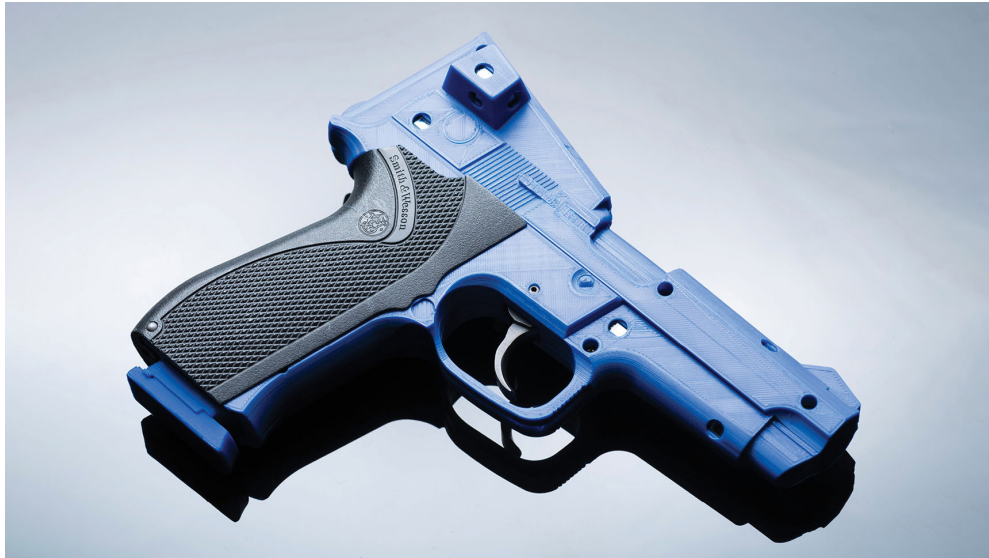
Figure 6. SteamVR HDK based 3D Printed Pistol
