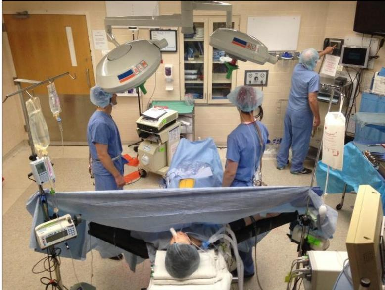
**Figure 1.** A photo taken during early system testing. The wet electrode EEG cap is worn under the surgical bonnet. A flat ribbon wire transmits the EEG signal to the BioRadio sensor, which is attached to the participant's belt. ECG data is collected via electrodes that are attached to the chest.
