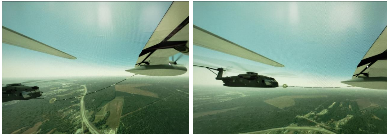
Figure 2. Receiver Aircraft at Astern and Contact Position
