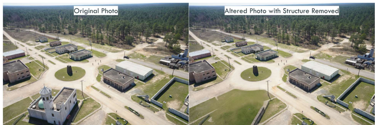
Figure 8. To test the reductive case, an image was altered to make it appear that the building was removed. This was then used as an input for sparse-view reconstruction.
