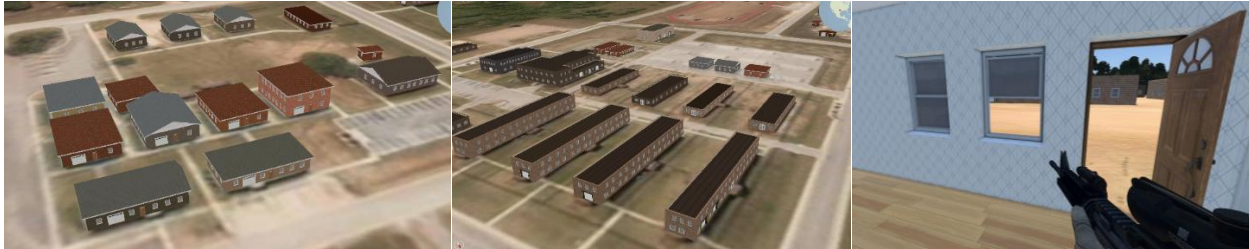
Fig. 10. Buildings from floorplans created by the Floorplan Architect Tool from 2D footprints
