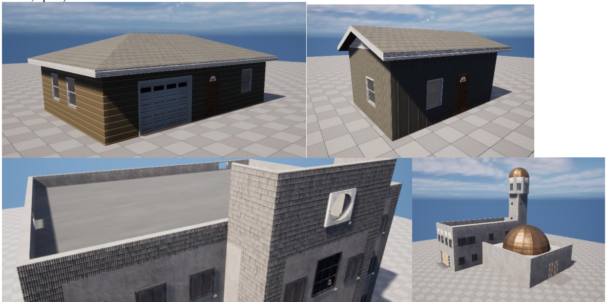
Fig. 7. (Top Left) BFF with hip asphalt shingle roof with white painted wood fascia (Top Right) BFF with gable roof using same defined assets. (Bottom Left) Flat concrete roof with parapets (Bottom Right) BFF with flat roofs and dome models
