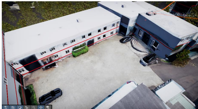
Figure 5. Building models, with "window-holes" that were "dug" out of the original building model, were populated with window structures and marked by floor with red lines.
