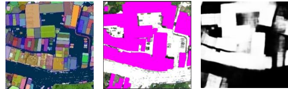
Figure 12. Building-related SAM mask (left), ground truth masks (middle) and classification masks (right)
