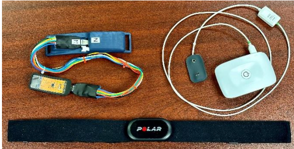
Figure 2. Participants wore two fNIRS sensors (MAVERIC, top left; Pioneer, top right) and one heart rate chest strap (bottom).
