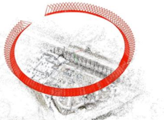
Figure 9. Visualization of bundle adjustment process running in the COLMAP GUI. Each camera location (red triangles) is being refined and placed showing our circular flight path around the scene with corresponding sparse reconstruction (colored dots).
