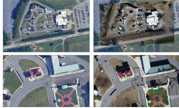
Figure 11. Safety Park scene with pre-existing image basemap and drone locations overlaid with red dots (top left), orthomosaic rendered from QuickView NeRF (top right), zoom in of town square (bottom left) and updated zoom in with NeRF based render (bottom right). Notice the absence of tilted buildings / structure in bottom right NeRF based orthomosaic.
