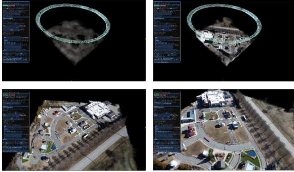
Figure 10. Generating a QuickView product using InstantNGP to train and display a NeRF of the Safety Park scene. Initial training (top left), converging model (top right), and two new views of the scene (bottom left / right) all occurring in a few seconds.
