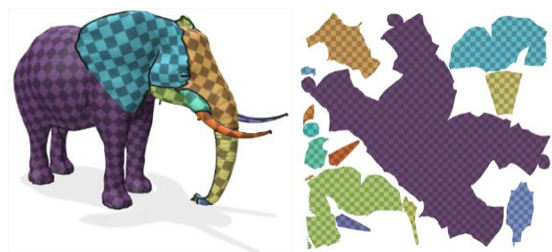
Figure 22. A complex 3D mesh (left) and a corresponding 2D parameterization (right).
