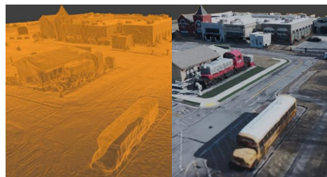
Figure 17. Original mesh produced by Neuralangelo with (left) and color information (right).
