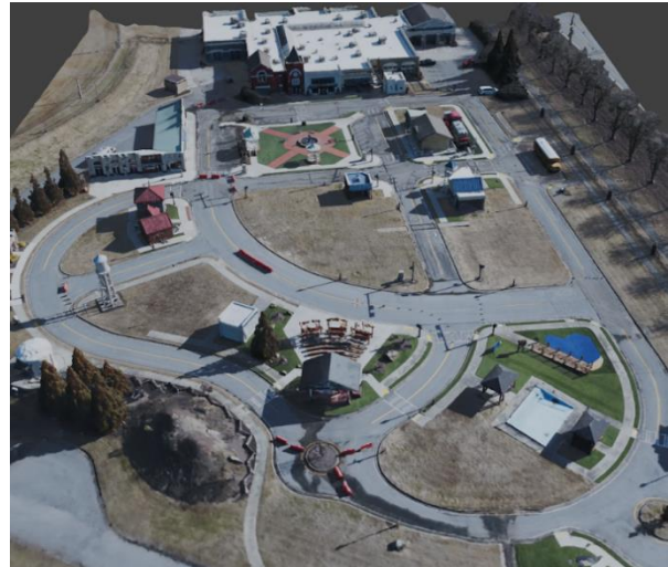
Figure 1. Example surface mesh extracted from a series of overlapping drone images of Safety Park, a first responder training facility in Atlanta, GA. This is viewed within the popular open-source tool Blender and is of suitable quality for creating a digital twin of the facility.
