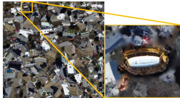
Figure 24. On the left, the texture generated by transferring vertex colors to a texture image based on the mesh parameterization produced by AutoUV. On the right, a subset of the texture focusing on the school bus.
