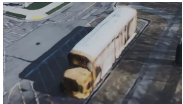
Figure 21. Top-down mesh parameterization causes loss of color detail in vertical geometry.
