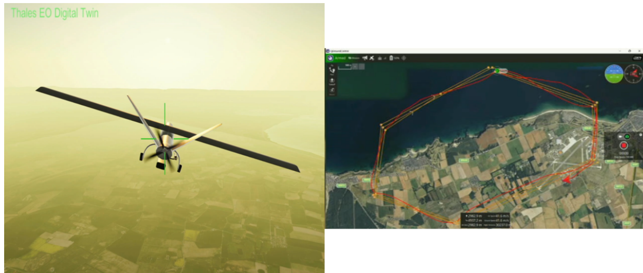
Figure 7: Snapshot from UAS Digital Twin from the Thales Training and Simulation (TTS) Digital Twin Image Generator (IG), live in deployment (right). Q Ground Control Service acting as the platform ground control; visualizing the waypoints for the DT to fly to, as well as the historical flight path.
