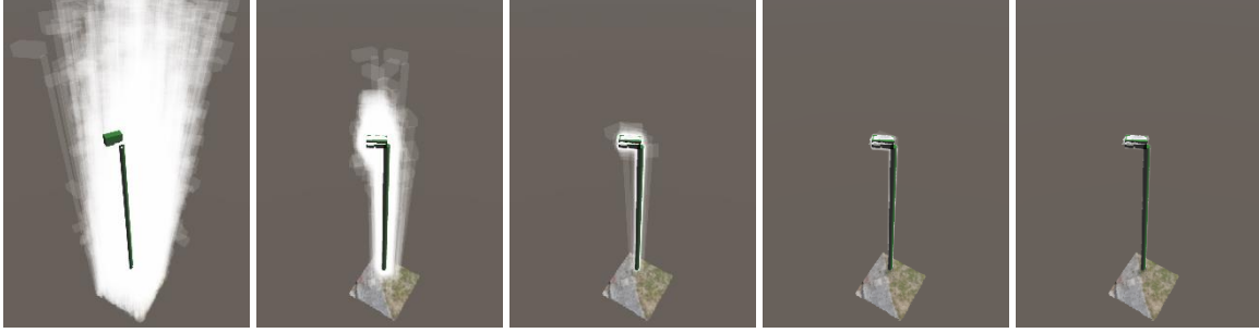
Figure 8. A visualization of how APSO finds a solution for the light pole model in POLE1, from the first iteration (left), to the state where all particles converged (right). Iterations 0, 10, 50, 100 and 200 are shown. In white a subset of the individual particles, in green the current best solution.
