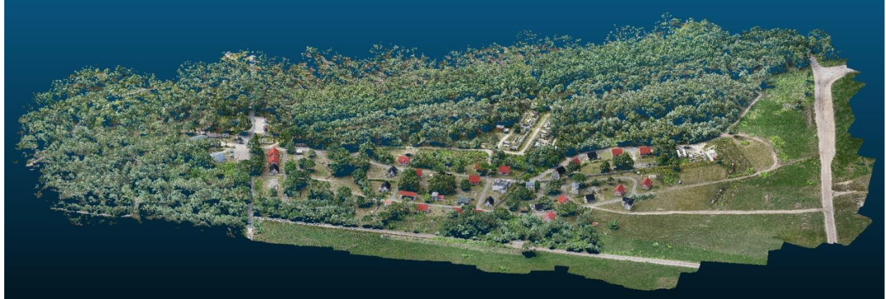
Figure 4. The test data set: a photogrammetrically derived high resolution point cloud of a military training village.
