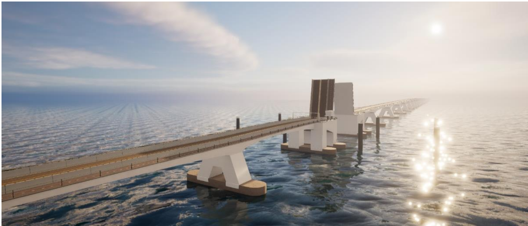
Figure 3. A procedural bridge model, automatically generated from terrain elevation data and a linear vector describing the location and configuration of the bridge. Generated with Houdini, exported to and shown here in Unreal Engine.
