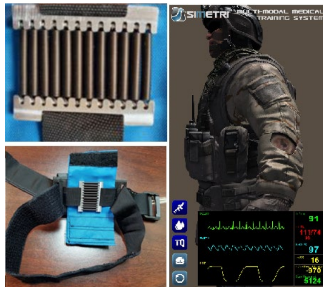
Figure 1: Surrogate Tourniquet Modified with Force Feedback System (left) and Mobile App Screen (right)
