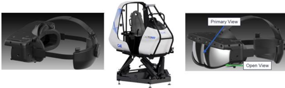
Figure 1 – JVC S1 high-fidelity optical head-mounted display on a motion device with flight control and cockpit replica
