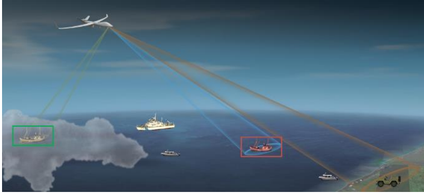
Figure 4. Warfighter uses ATR model on live field data, data is collected and sent back to rapid retraining process to improve model performance
