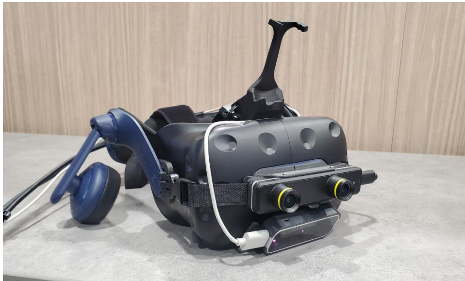
Figure 2. HTC Vive Pro 2 Hybrid XR headset with ZED cameras and UltraLeap
