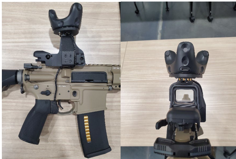
Figure 6. Trigger System and Red Dot Sights with Custom Mounted Tracker
