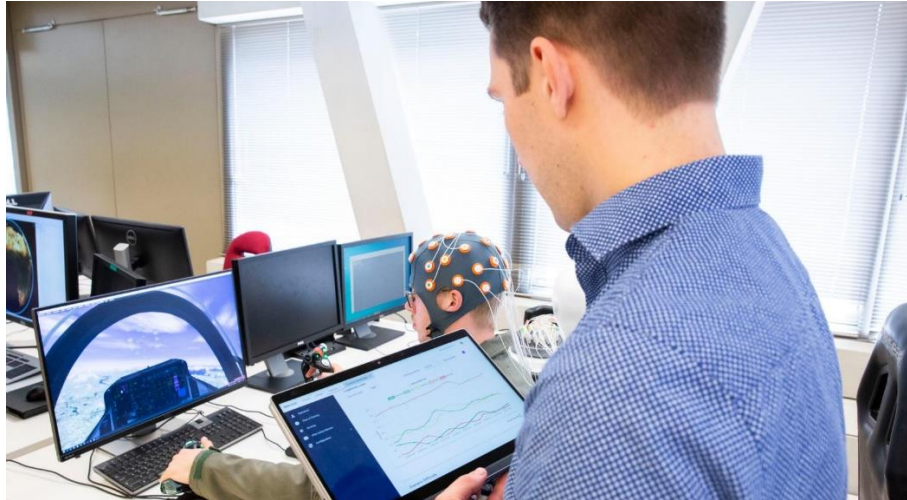
Figure 4 Desktop simulator controlled with operator that is wearing an EEG to measure cognitive load, which is visualized to the instructor
