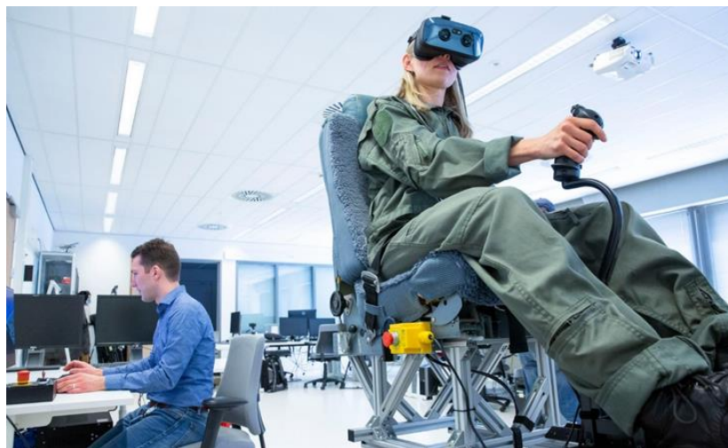
Figure 3 Motion Based VR Simulator
