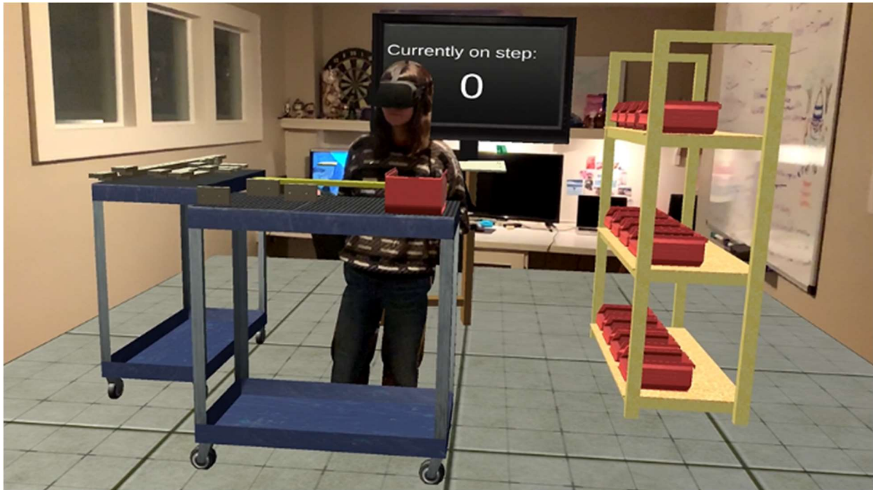
Figure 5. A view of the final AR application showcasing both the AR digital twin and body occlusion. The trainee is wearing a VR Oculus Quest 2 HMD
