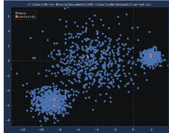
Figure 10 – Correlated Histograms applied to varied. Number of QRDE bins = 42, 32 for x, y respectively, sensitivity = .9.
