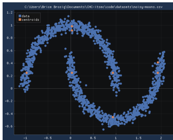
Figure 11 – CHC applied to the noisy-moons dataset with sensitivity = .90 and bin count for QRDE set to 100 for both x and y.
