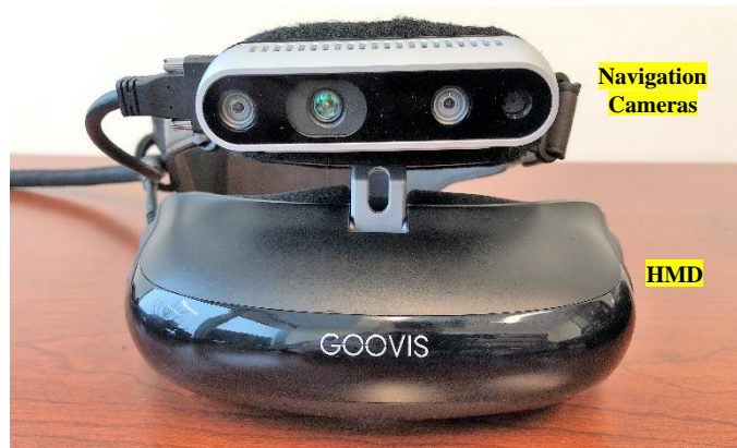
Figure 3. The HMD and navigation cameras
