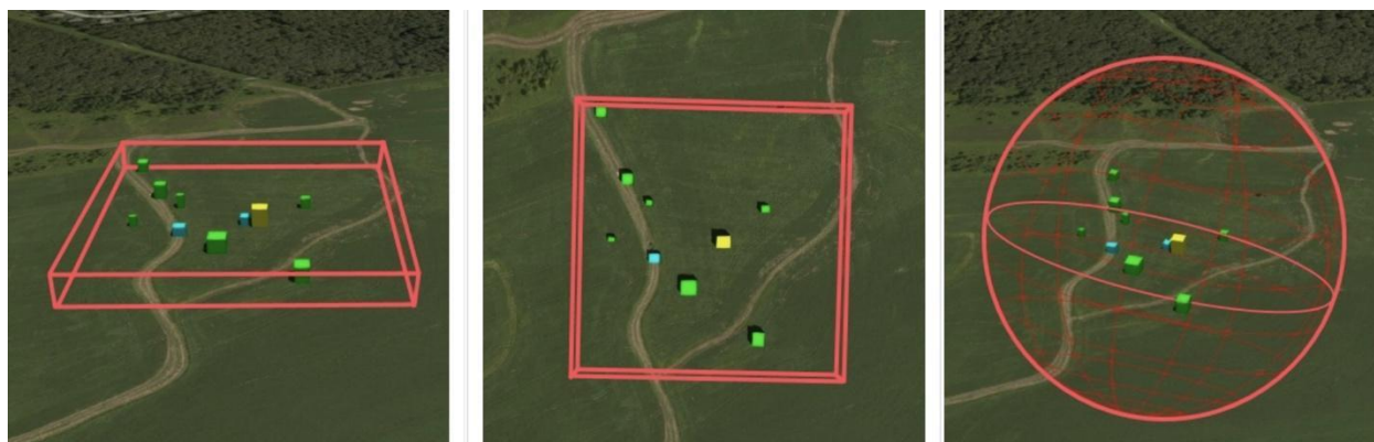
Figure 3: Bounding volumes: Box (left), region (convex hull, middle), sphere (right)
