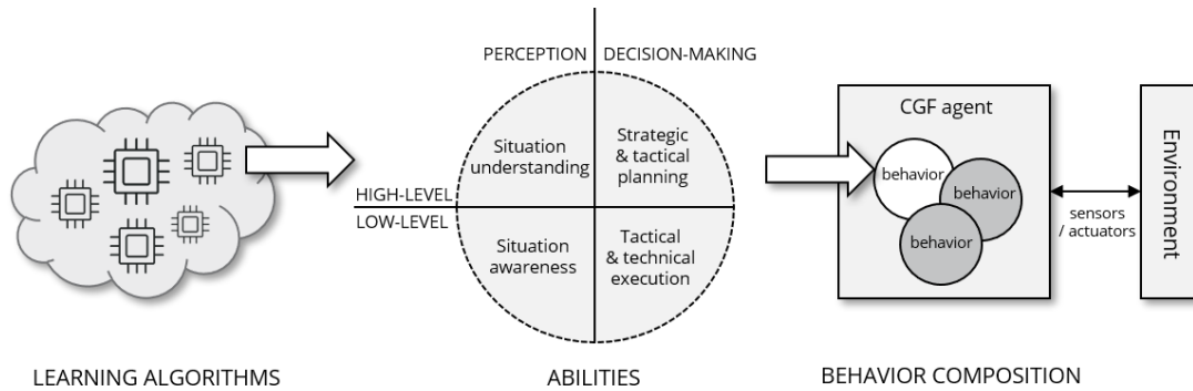
Figure 2. Conceptual CGF Design: Learning algorithms (left) fulfill behavioral abilities (center) that are composed to form a CGF (right).
